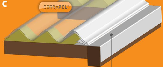
STRAIGHTEN and LOCK the CORRAPOL® Rock n' Lock Side Flashing into place giving a perfect finish to the edge of your roof structure.
